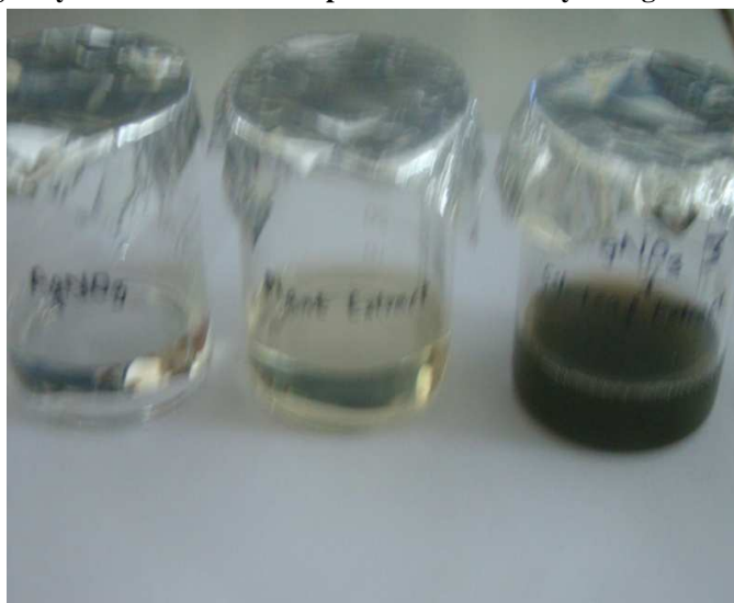
Fig. 1 Synthesis of silver nanoparticle indicated by change in colour
